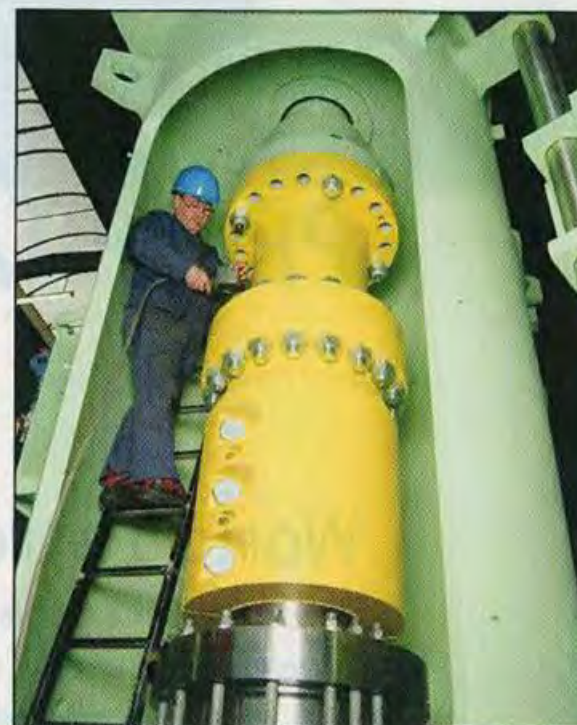
FIGURE 1. This drive-shaft coupling and mechanical seal are for an 800-m 3 gas-liquid reactor
